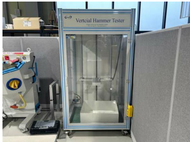
Vertical Hammer Tester
