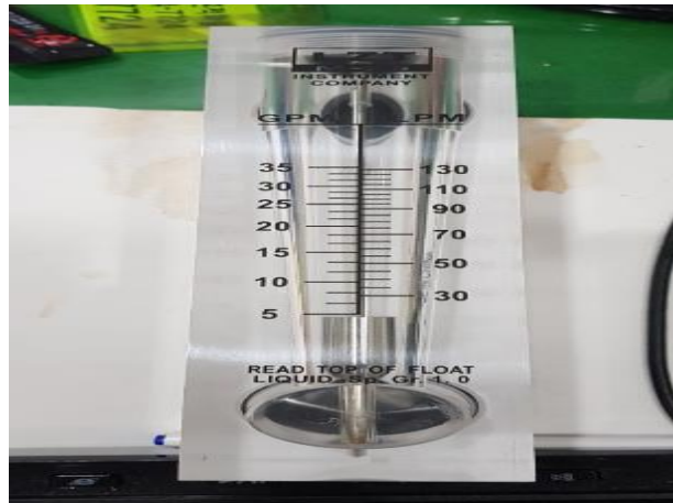
Water flow meter with IPX6
