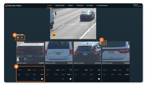
To activate the display of the events as tiles, click A button. In this mode events and their parameters (Date/Time, Plate, Direction, Photo, Country, Type, Brand, Model and Color) are displayed in tiles.
