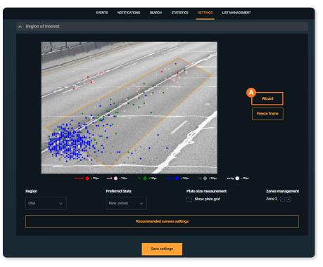
(A) Wizard tool displays the statistic on location and sizes of the latest 1000 recognized plates.
